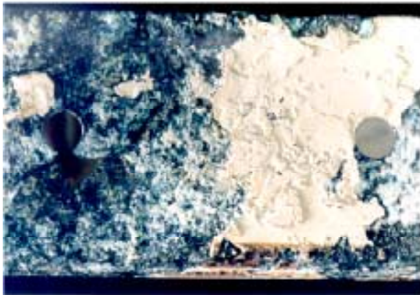
Aircraft aluminum corrosion
